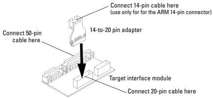
**3** Connect the other end of the 14- or 20-pin cable to your target system.
